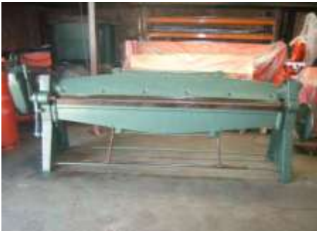
EDWARDS Cast Hand Operated Straight Folder 'Highlift' 8ft x 14swg Capacity. Lift Height: 6" (150mm)
