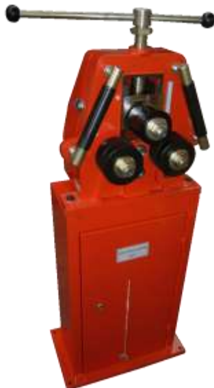
Ring Roller. Flat Bar: 25mm wide x 3.0mm Thick - min. Ring Diameter 75mm Round Bar: 7.0mm Diameter - min. Ring Diameter 75mm. (RR25). Price: £95.00.
