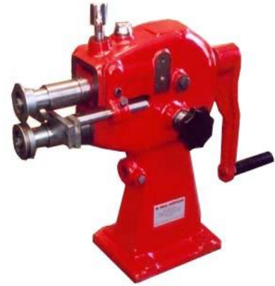
WNS Hand Swager 215mm Throat x 1.2mm Capacity. (HS215)
