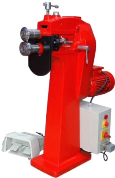
WNS Power Swager 280mm Throat x 2.0mm Capacity. (PS280)
