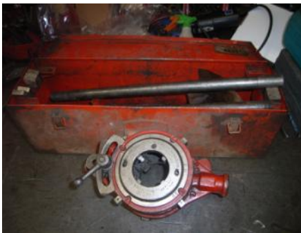
PRESTO Hand Threader Ratchet & Die Set 1150R. 2" BSP/13 1/2R. 22" Long Handles. Chasers: 1/4, 1 1/2 & 1/2.
