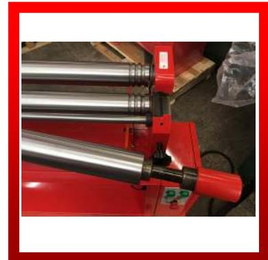
**WNS POWER BENDING ROLLS (PBR1300/75)** are principally used for rolling tubes/cylinders in sheet metal. The metal is 'pinched' between two rolls and curves as it comes into contact with the third (back) forming roll. The PBR1300/75 has a 1300mm Rolling Length, 75mm Roll Diameter and can accommodate Mild Steel up to 1.5mm thick. The rolls are top slip, equipped with 3 wiring grooves and the Back Roll is Adjustable for (limited) coning.
