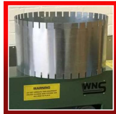
**WNS EDGE NOTCHERS (EN20)** are the ideal machines for air conditioning and ductwork applications. They are principally used for punching slots into the edge of sheet metal to produce collars for ductwork, ductwork fittings and end caps. The material is driven through the punching head by two powered rolls, progressively notching the edge of the metal with precision and accuracy.
