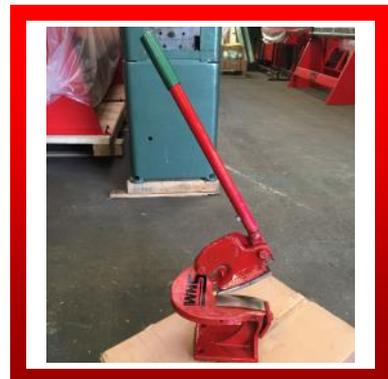
**WNS THROATLESS SHEAR (TS100H)** is designed for cutting steel sheet and/or flat steel. The machine has a 100mm blade and can accommodate mild steel sheet up to a maximum of 1.5mm thick. This machine has adjustable blades and burr free cutting.
