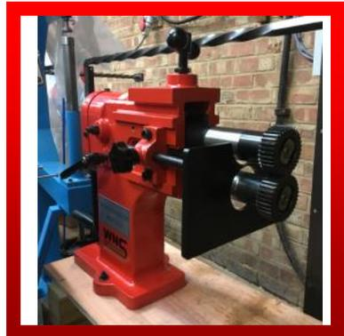
**WNS HAND SWAGERS (HS200)** are principally used for swaging, beading, wiring, crimping and forming of sheet metal. This Hand Swager has a 200mm (8") throat and can accommodate mild steel sheet up to a maximum of 1.2mm thick. This machine comes complete with 5 sets of rolls.
