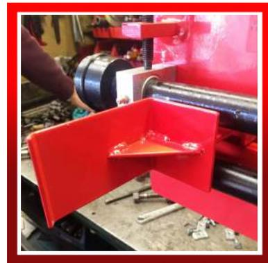
**WNS BEAD ROLLER ADJUSTABLE GUIDE FENCE (BRGF)** assists in creating even, straight beads along your piece of metal. This tool is compatible with WNS Bead Rollers BR457, BR464HD & BR305H. This Guide Fence may also be suitable for other brands of Bead Rollers.
